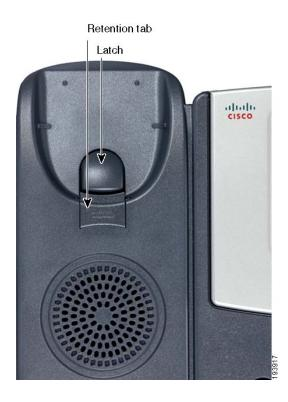
STEP 3 Rotate the tab 180° and re-insert into the phone base. The tab now catches the slot in the handset when the handset is placed onto the cradle.
